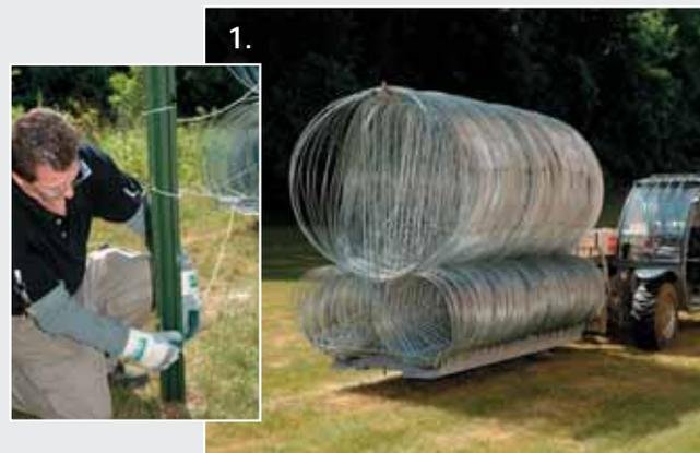
**1. SET** Set the RDU in place using any vehicle with fork attachments. A trailer option is available.
